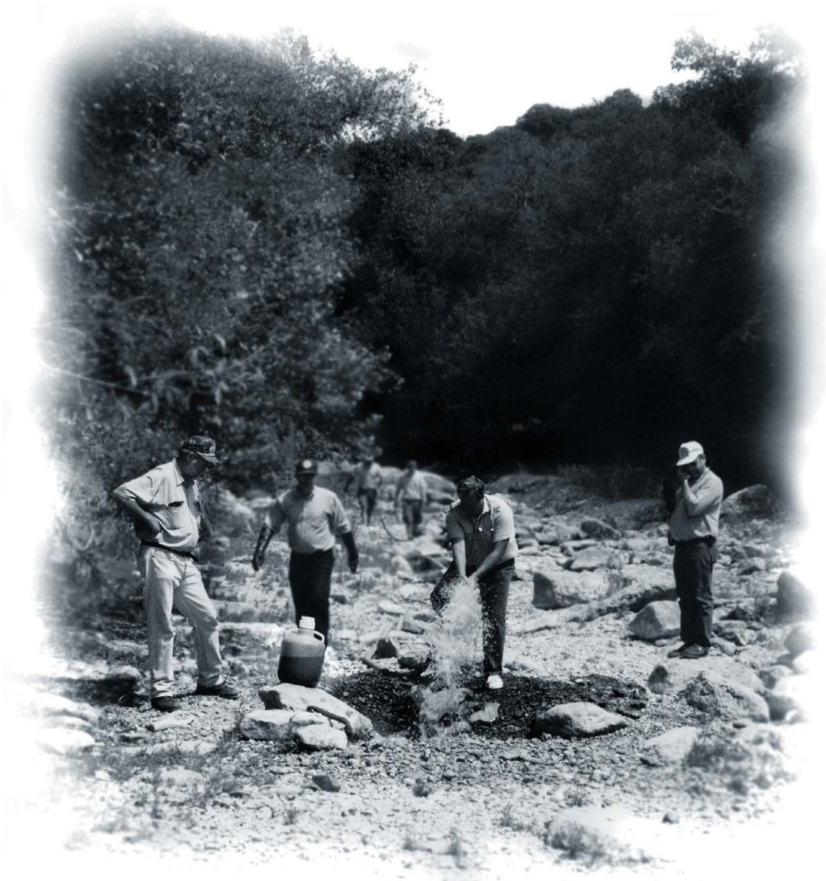
Introducing water and fluorescein dye into a sinking stream point, Edwards Aquifer, Texas. Note the dye and water mixture in the 20-liter carboy.
