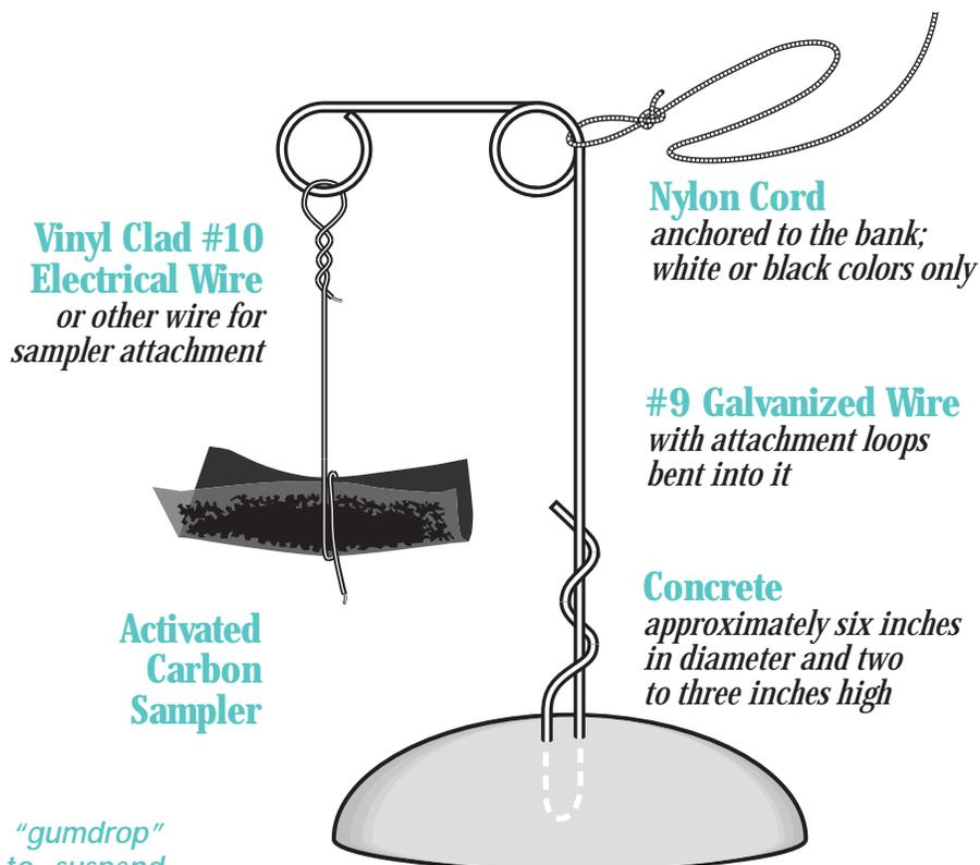
**Figure 3** A "gumdrop" sampler used to suspend activated carbon samplers above the stream bed.
