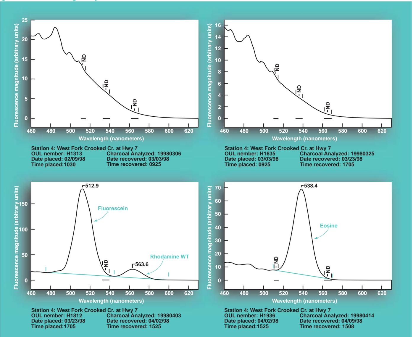
**Note** The top two graphs show no detectable dyes. The graph at bottom left shows fluorescein and rhodamine WT. The graph at bottom right shows eosine only. Please note the different scales on the Y-axis.
